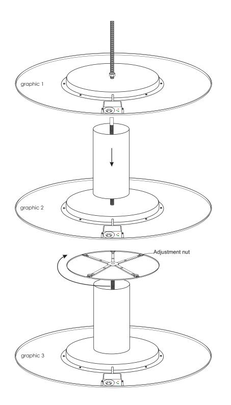
**Step 1:** Open the box/remove lid. Tabletop is laying bottom up in the box. Remove packaging from threaded rod (packed separately).
